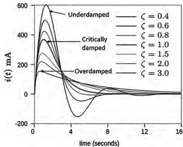
**Figure 3.10.** Underdamped, overdamped, and critically damped circuit responses for varying values of  $\zeta$
