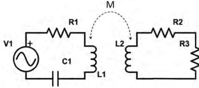
**Figure 3.14.** In this WPT system, the left circuit has a capacitor while the right circuit does not have one. It is modeled by a system consisting of one second-order and one first-order differential equation.
