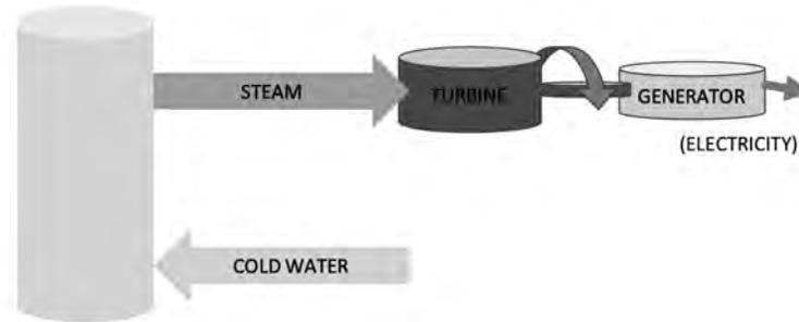
**Figure 3.15.** Block diagram of a nuclear power plant. One of the things mechanical engineers have to do is design the system so that the steam retains its heat before going to the turbine. This improves the efficiency of the system.
