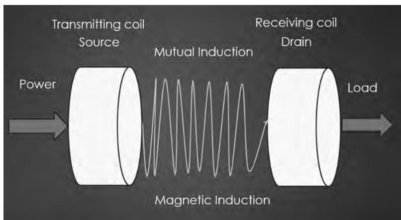
**Figure 3.11.** A schematic diagram of a WPT system
