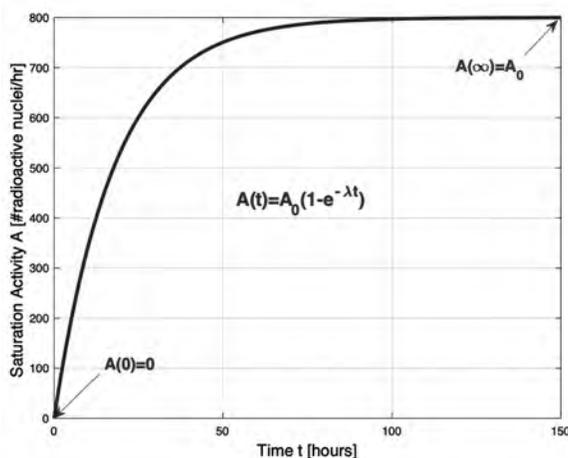
**Figure 3.21.** Representative curve showing the saturation activity  $A$ , which converges exponentially to the rate of nucleus production,  $A_0$ .
