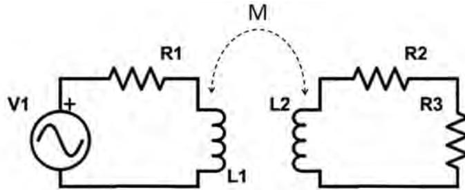
**Figure 3.13.** In this WPT system, both circuits do not have capacitors. It is modelled by a system of two first-order differential equations.
