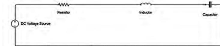
Implement the circuit shown in online simulator (PartSim or Simulink) and observe the voltage across capacitor in simulations.
