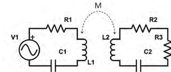
**Figure 3.12.** A WPT system consists of two circuits coupled by a mutual inductance
