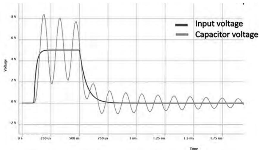
3. **Circuit 2:** Use  $R = 200\Omega$ ,  $L = 2.2mH$ , and  $0.22\mu F$ .
