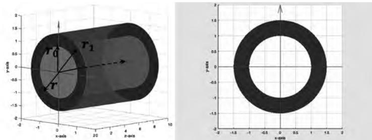
**Figure 3.16.** (left) General 3-D view of an idealized pipe used to carry heated fluid from point A to point B. (right) Cross-sectional view.
