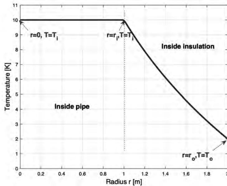
**Figure 3.20.** The distribution of  $T$  along the radius of the pipe insulation. Internal heat is assumed constant.
