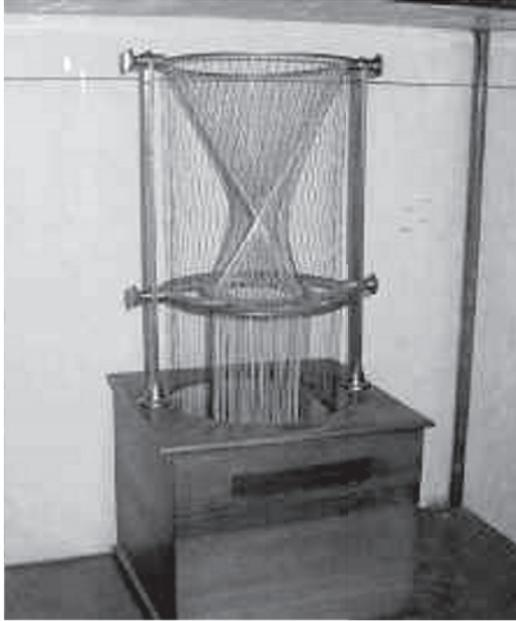
Figure 2. Cylinder and Hyperboloids.
